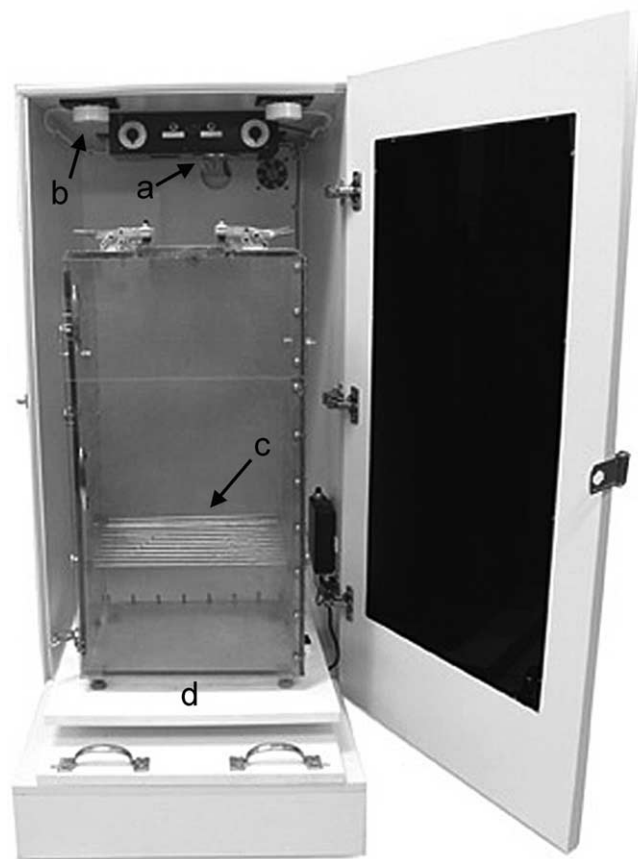
Figure 1. A photograph of the fear-potentiated startle apparatus (Med Associates). Arrows point to the speaker assembly ( a ), to one of the four ceiling lights ( b ), and to the floor of the chair ( c ), which has adjustable levels for different monkey heights. The load cell/strain gauge ( d ) is located under the upper panel of the platform. The animal is transferred in a custom-built primate restraint chair that is positioned on the platform and secured with side wing nuts.
