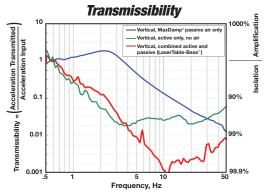
TMC's two-tiered LaserTable-Base<sup>™</sup> combines a patented MaxDamp<sup>®</sup> Gimbal Piston<sup>™</sup> air vibration isolation system to isolate high frequencies and the patented STACIS<sup>®</sup> technology incorporating piezoelectric actuators and inertial
