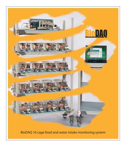
If you are using any other method for ad libitum food intake measurements you are only scratching the surface. The BioDAQ Food & Water Intake Monitor records the native *episodic* intake behavior of rats and mice at very high resolution in their home cage.
