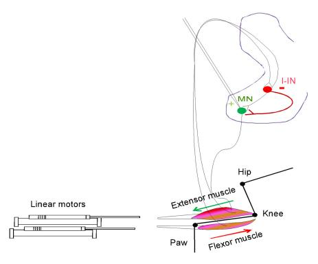
**Figure 4.** Illustration of the computer-controlled linear motor set up to test the push—pull hypothesis within cells. The distal tendons to ankle extensor and flexor muscles were attached to the linear motors, which independently controlled muscle lengths while measuring effective synaptic currents in ankle extensor motoneurons. I-IN, Inhibition from inhibitory interneurons.
