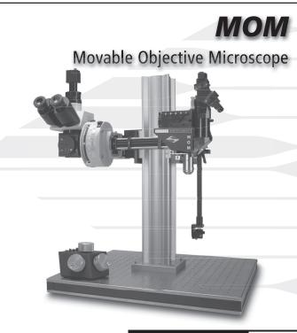
The Movable Objective Microscope (MOM) is a two-photon microscope capable of imaging deep within living specimens when combined with a Ti:Sapphire laser. The MOM design is unique in providing 3-dimensional objective movement and rotation allowing the specimen to remain stationary.
