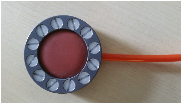
Figure 1. Device for sensory-tactile stimulation of the clitoral region and dorsum of the right hand. The stimulus is delivered via a noninvasive air-controlled oscillating membrane with a compression of \sim 0.1 bar.
