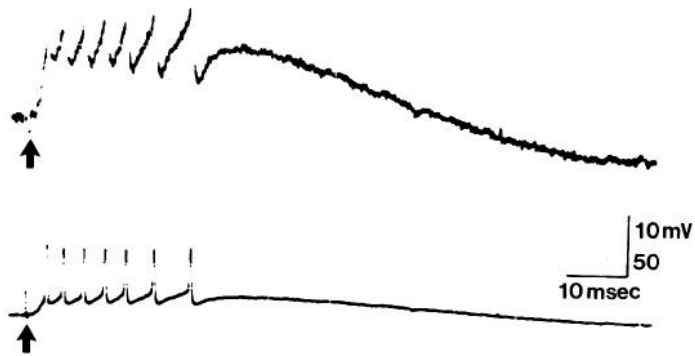
Figure 1. Typical intracellular record from a neuron in the somatic sensory part of the reticular nucleus, showing the large EPSP and train of spikes ensuing following a single 28-V, 20- \mu sec electrical shock (arrow) applied to the arm area of the ipsilateral somatic sensory cortex. Upper trace, High gain AC; lower trace, low gain DC.
